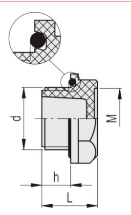
$\begin{array}{lll} d & = M \ 16x1.5 \\ D & = 25.5 \\ h & = 10 \\ L & = 18 \\ M & = 17 \\ s & = 22 \end{array}$
